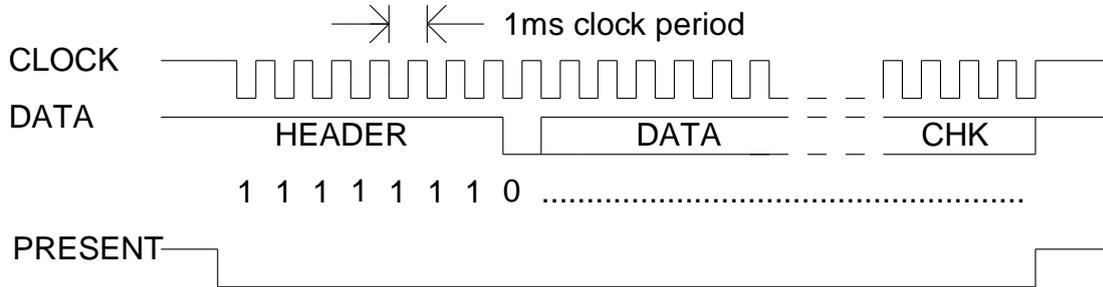
Data is set up on the falling edge of the clock and is stable on the rising edge of the clock.
