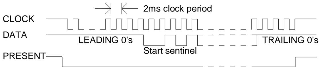
Each character is 5 bits long. The first four bits are the hex digit (0-F) least significant bit first. The fifth bit is an odd parity bit. A 0 is represented by a high level on the DATA connection and a 1 is represented by a low level on the DATA connection. Data is set up on the falling edge of the clock and is stable on the rising edge of the clock. The PRESENT output goes low for the duration of the transmission simulating the CARD PRESENT from a mag card reader.
