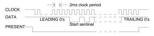
Each character is 5 bits long. The first four bits are the hex digit (0-F) least significant bit first. The fifth bit is an odd parity bit. A 0 is represented by a high level on the DATA connection and a 1 is represented by a low level on the DATA connection. Data is set up on the falling edge of the clock and is stable on the rising edge of the clock. The PRESENT output goes low for the duration of the transmission simulating the CARD PRESENT from a mag card reader.
