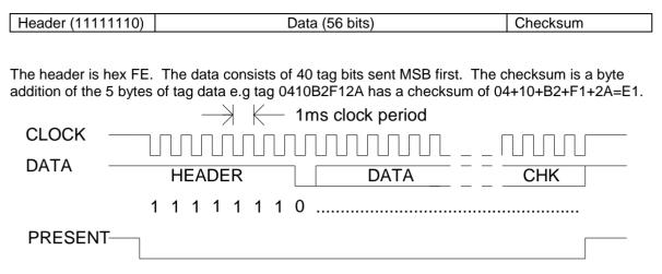
Data is set up on the falling edge of the clock and is stable on the rising edge of the clock.
